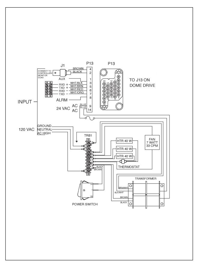
Figure 3. 120 VAC Back Box Wiring Diagram
